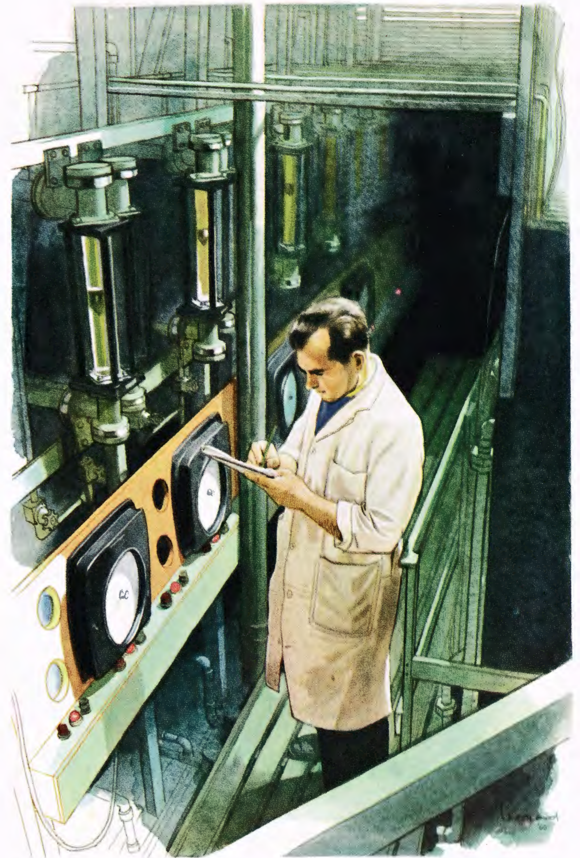
Control bridge. Keeping a careful watch on the control instruments, this process worker checks solution temperatures and rates of solution flow. If they are wrong, he makes the necessary adjustments
